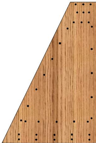
Left side roof panel, topside, showing screw patterns
